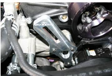
6. From the rear and below the compressor case, insert the slide bracket into the bracket slot.
